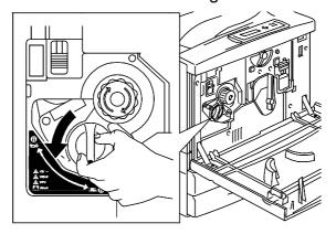
4. Pull the Toner Cartridge out of the Printer.
