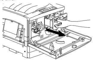
6. Grasping the **handle**, remove the cartridge from the Printer. Ensure that the cartridge remains level.
