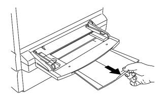
5. Insert your paper stock into the Bypass Tray. Place the left-hand edge of the paper stock against the left-hand paper guide.
