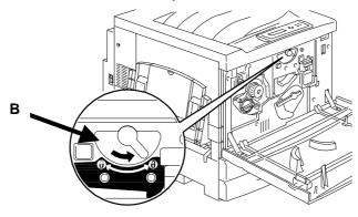
5. Place your fingers into the opening on the front of the Print/Copy Cartridge and pull it slowly toward you. DO NOT remove it from the Printer at this time.
