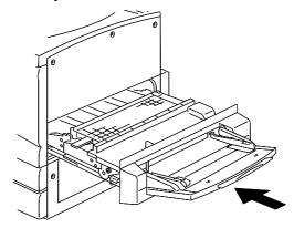
8. Reload the Bypass Tray with the desired stock and ensure that the width guide is adjusted to the size of the stock.
