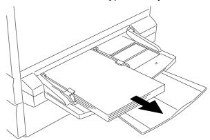
3. In order to access a jam in the transport, pull the Bypass Tray all the way out of the Pinter.
