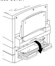
2. Remove any jammed or torn stock from Area 2. Ensure that there are no pieces of torn stock remaining in the area.
