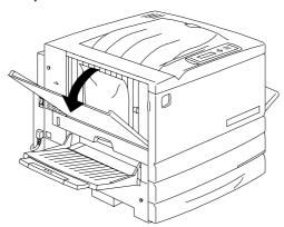
2. Remove the jammed paper. If the paper is torn ensure that there are no pieces of torn paper remaining in the Printer.
