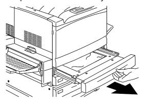
2. Remove the jammed paper and any paper that is creased or torn. Ensure that there are no pieces of torn paper remaining in the tray.
