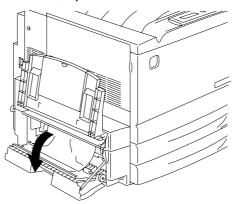
2. Remove the jammed paper. Ensure that there are no pieces of torn paper remaining in the Lower Inverter.
