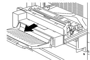
2. To release any paper, lift the **Green Lever**, and gently pull the paper in the direction of the arrow. If the paper is not visible, turn the **Green Knob** in the direction of the arrow.
