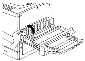
5. Remove any jammed or torn paper as shown below. Ensure that there are no pieces of torn paper remaining in the transport.
