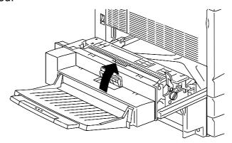
a. If paper is visible under the clear cover, hold the cover open and push the paper toward the paper exit with your fingers.
