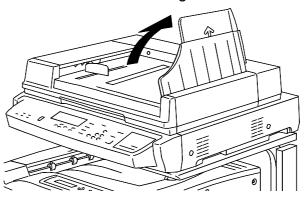
2. Place the originals into the ADF face up and in the same orientation as the paper in the Paper Tray.
