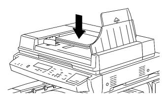
3. Gently push the originals into the ADF, as shown below, until the ADF Light illuminates.
