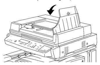
6. If you are loading large size originals into the ADF, pull out the Exit Tray Extension of the Document Exit Tray.
