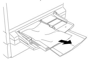
2. Remove any stock loaded in the Bypass Tray.
