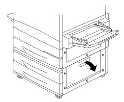
2. Remove any jammed or torn paper as shown below. Ensure that there are no pieces of torn paper remaining in the feed area.
