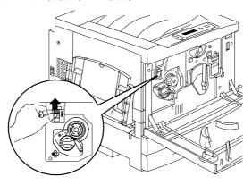
b. Turn the **Rotary Knob** in the direction of the arrow until it stops.
